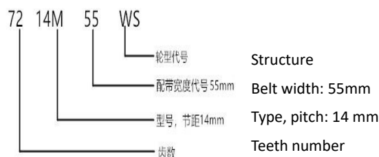
同步带轮基本形状结构图例/Timing belt pulley structure legend
